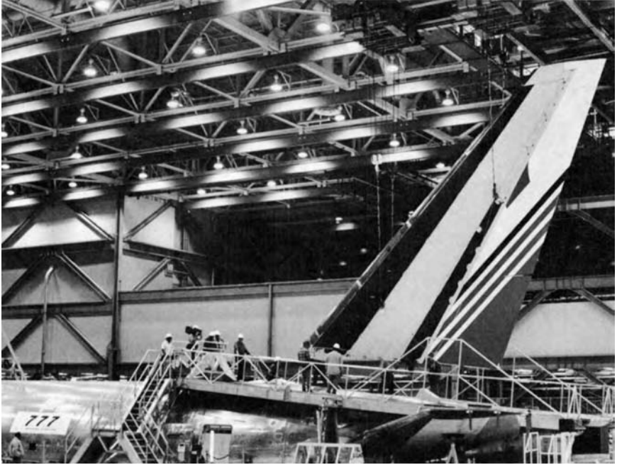
FIGURE 5.1 The first carbon matrix composite vertical stabilizer for a Boeing 777 jet liner is hoisted into position. (Courtesy of Boeing Commercial Airplane Company. With permission.)
