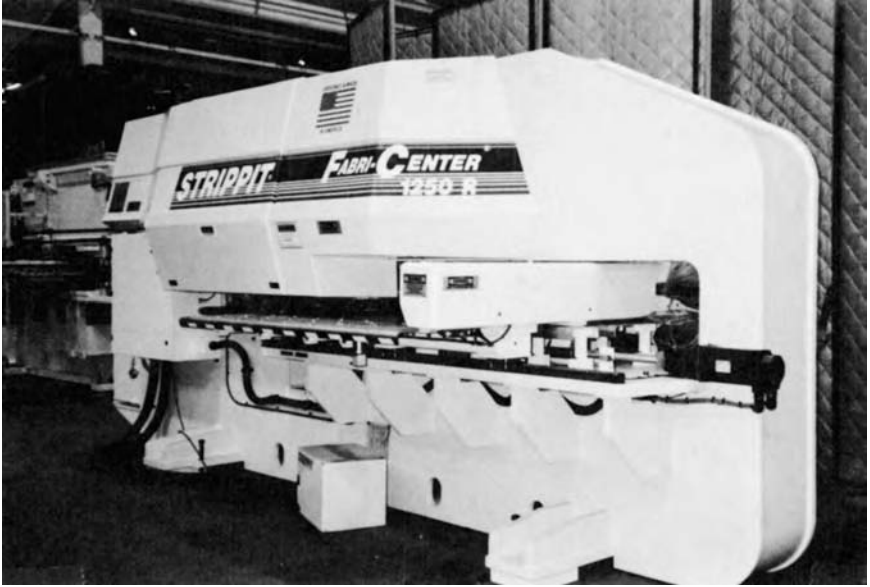
FIGURE 3.5 Example of a turret punch. (Courtesy Strippit, Inc. Akron, NY. With permission.)
