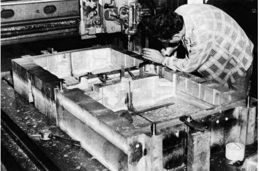
FIGURE 5.6 A tool maker works on the cavity of a large mold. (Photo courtesy of SPL.)
